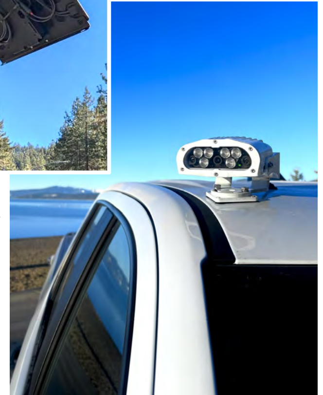
Vehicle-mounted LPR Unit in Placer County
