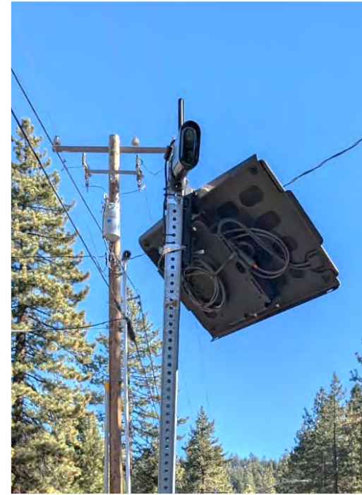
Fixed-mount LPR camera in Douglas County
