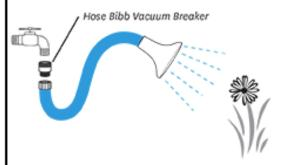
sure that no harmful materials are drawn back into the garden hose, a vacuum breaker should be installed on each hose bibb. When the hose bibb is exposed to freezing conditions, make sure to use a self draining, frost-proof vacuum breaker.
