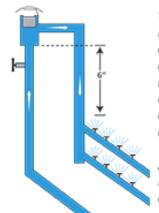
Vacuum Breakers must be installed above ground and above all sprinkler heads--a minimum of 6" for an AVB and 12" for a PVB and SVB
