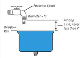
separated or "air-gapped." If there is no airgap, then the contents of the sink, tub, or tank may be sucked or "backsiphoned" into the water line during a loss of water pressure.
