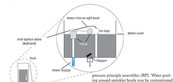
the correct type so that the contents of the toilet tank don't get back into the drinking water system in your house. As shown in the illustration, the anti-siphon ballcock and refill tube must be above the water level in the tank.
