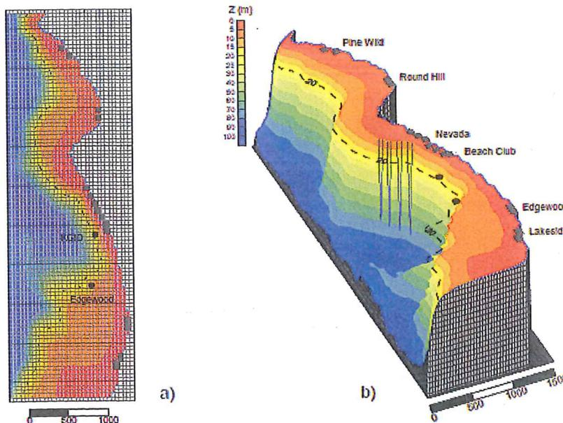
Fig. 3.1. Bathymetry and segmentation for the numerical model for the Kingsbury Grade and Edgewood water intakes. a) bathymetry represented as contour plot with computational grid overlain; b) bathymetry represented as wireframe with beaches identified.
